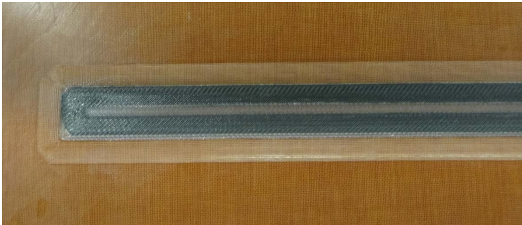
Figure 19. A Close-Up View of the Continuous Carbon Fiber Composite Still on the Print-Bed after Printing
